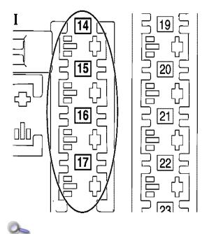
Incorrect numbering of the IEC Bus bar (Picture II)
